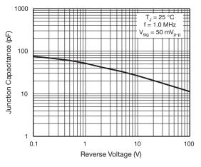
Fig. 5 - Typical Junction Capacitance
