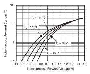
Fig. 3 - Typical Instantaneous Forward Characteristics
