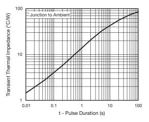
Fig. 6 - Typical Transient Thermal Impedance
