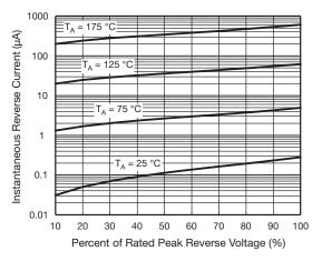
Fig. 4 - Typical Reverse Leakage Characteristics
