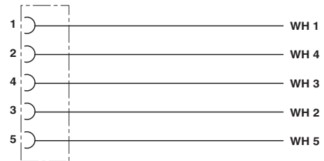
Contact assignment of the M12 socket
