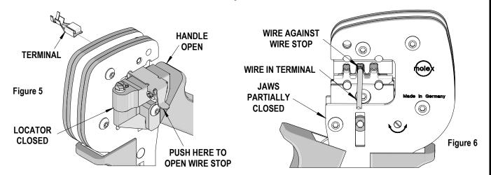
3. Swing the terminal locator away from the crimp tool shown in Figure 4. Some terminals with large insulation grips may interfere with the crimp tooling when swinging the locator into position. The terminal must then be loaded into the locator in the closed/crimp
