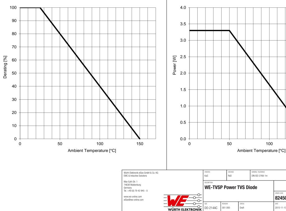
**Steady State Power Dissipation Derating**
