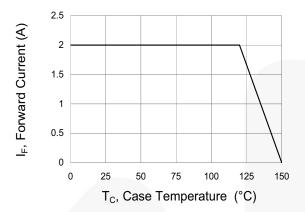
**Figure 1. Forward Current Derating Curve**
