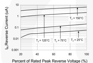
Figure 3. Typical Reverse Characteristics
