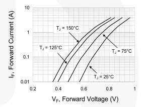
Figure 4. Typical Forward Characteristics
