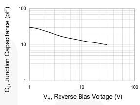
Figure 2. Typical Junction Capacitance
