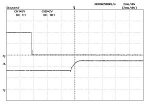
Figure 16: Turn on with Prebias 12Vin, 5V/0A out, Vbias =3.3Vdc
