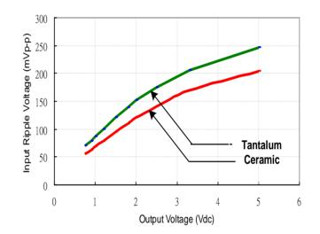
Figure 20: Input ripple voltage for various Output models, lo = 6A (Cin = 2x47uF tantalum capacitors and 2x22uF ceramic capacitors at the input)
