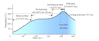
Note: All temperature refers to assembly application board, measured on the land of assembly application board.
