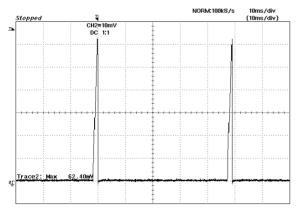
Figure 15: Output short circuit current 12Vin, 0.75Vout (5A/div)
