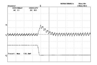
**Figure 13:** Typical transient response to step load change at 2.5A/μS from 100% to 50% of lo, max at 12Vin, 5.0V out (Cout = 1uF ceramic, 10μF tantalum) lo:2A/DIV
