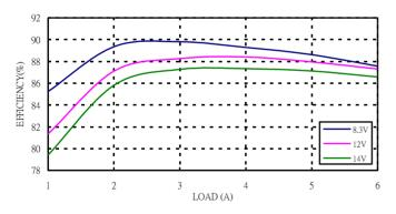
Figure 5: Converter efficiency vs. output current (2.5V output voltage)
