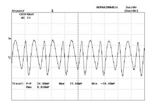
Figure 8: Output ripple & noise at 12 Vin, 2.5 V/6A out
