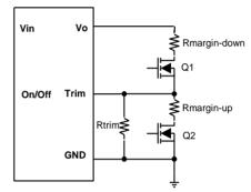
Figure 25: Circuit configuration for output voltage margining
