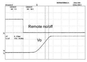
**Figure 12:** Turn on Using Remote On/Off with external capacitors (Co= 3000 μF), 5.0V/6A out
