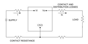
Figure 19: Output voltage and efficiency measurement test setup
