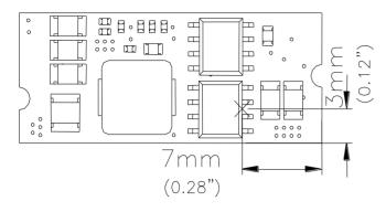
*Figure 31:* Temperature measurement location The allowed maximum hot spot temperature is defined at 115 C
