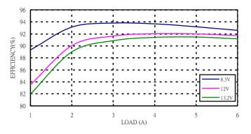
Figure 7: Converter efficiency vs. output current (5.0V output voltage)
