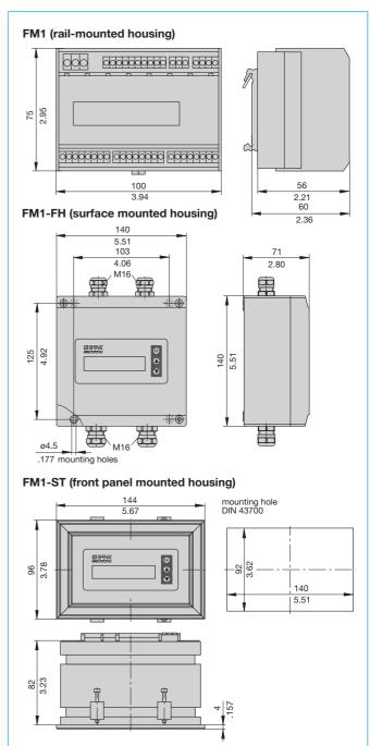
This is a metric design and millimeter dimensions take precedence ( $\frac{mm}{inch}$ )
