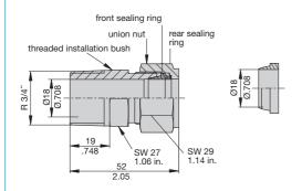
Suitable up to 25 bar/2.5 M Pascal if used with stainless steel CSF-01 monitoring head. (Observe instructions for installation.)
